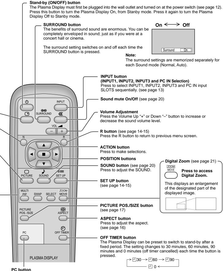
Press the "PC" input mode selection button to select the PC input mode.
